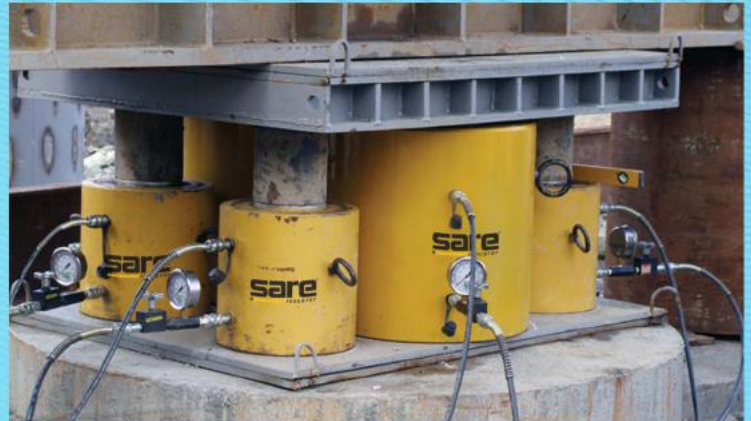
STATIC PILE TESTING JACKS
